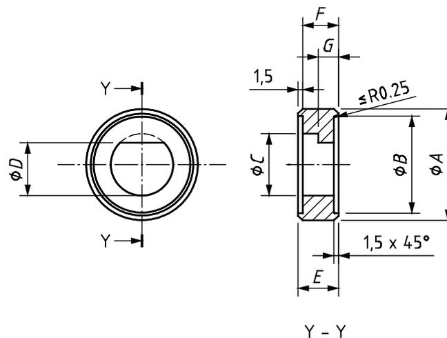
Machined surface roughness 3.2 μm all over
