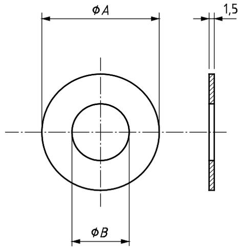
**Figure I.12 Gasket of a wafer type disturbance generator,
